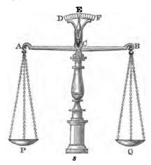
The annexed figure represents one variety of the Common Balance, which is an instrument for weighing bodies. It is essentially composed of a lever (AB) called a beam, which has a fulcrum (C) at its middle point, and two scale-pans (P and Q) suspended from its extremities.
